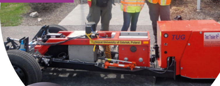
R2 Mk.2 test trailer for testing the rolling resistance of car tires during tests in the USA.
