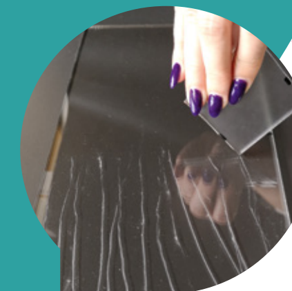
Photo on the left (upper part) - glass with a hardening coating (diamond-like). Photo on the left (bottom part) - glass without a coating.
